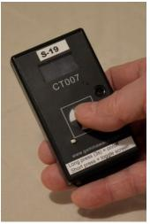
The CT007-S is a small general purpose survey meter type instrument that fits into the smallest pocket, without pinching the wearer. It uses the LND 713 GM tube, which is one of the standard tubes for this type of instrument. Its compact form factor and long battery life make it a convenient and easy to use survey meter.
